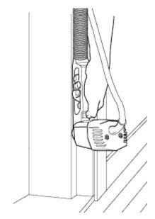
Then reverse the tool, starting at the center, and cut to the bottom.
