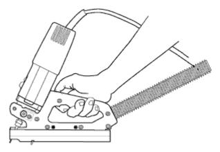
Push the button in the handle so that the standoff pin protrudes from the base.
