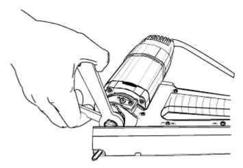
Insert the bit in the chuck so that it extends approximately 1/4" from the base and tighten the collet nut with the two wrenches provided.
