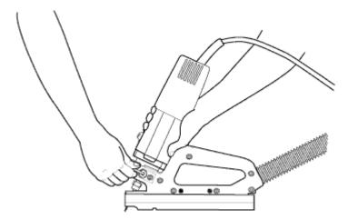
Loosen the clamping screw and turn the adjusting screw with the allen wrench provided.
